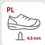
Durchtrittshemmung Textil (4,5 mm Nagel) Penetration Resistance Textile (Large Nail)
